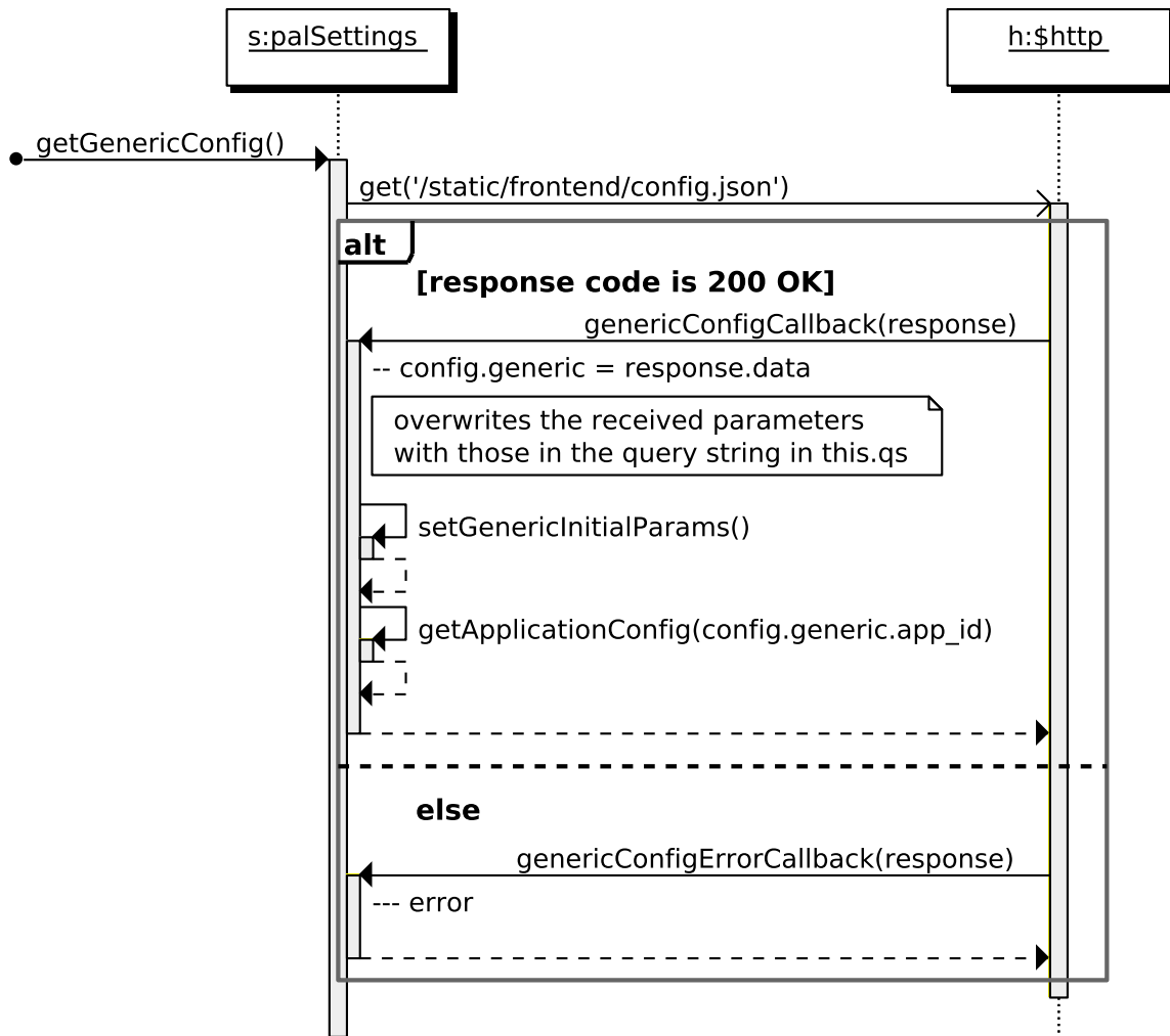
Figure 6-27: Sequence Diagram: getGenericConfig()
