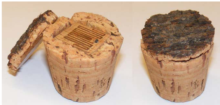
Figure 3.19: RFID tag inside a cork stopper. (left) - partial embedded and (right) - completely covered
