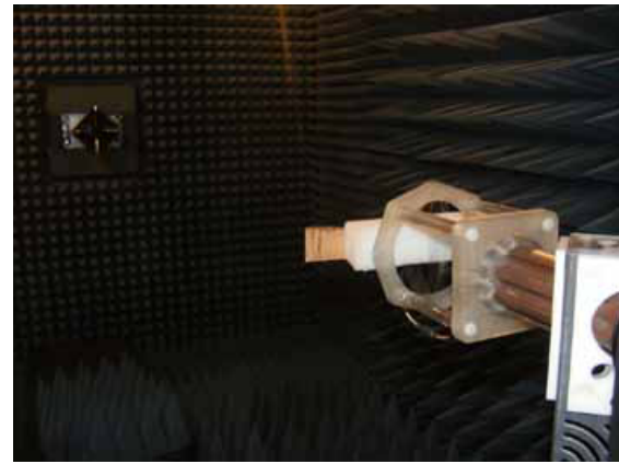
Figure 5.2: Photograph of the measurement setup in the anechoic chamber
