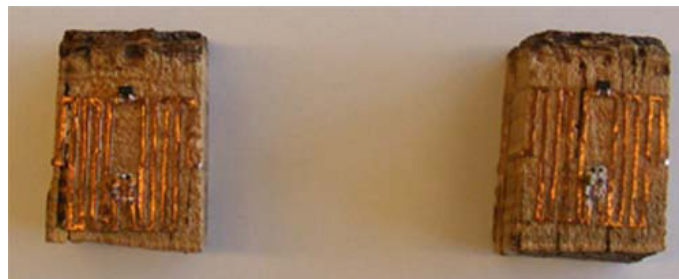
Figure 4.6: Two RFID tags with the implemented lumped network. The tag on the left has a resistance value of 100Ω and the tag on the right, a 150Ω resistance
