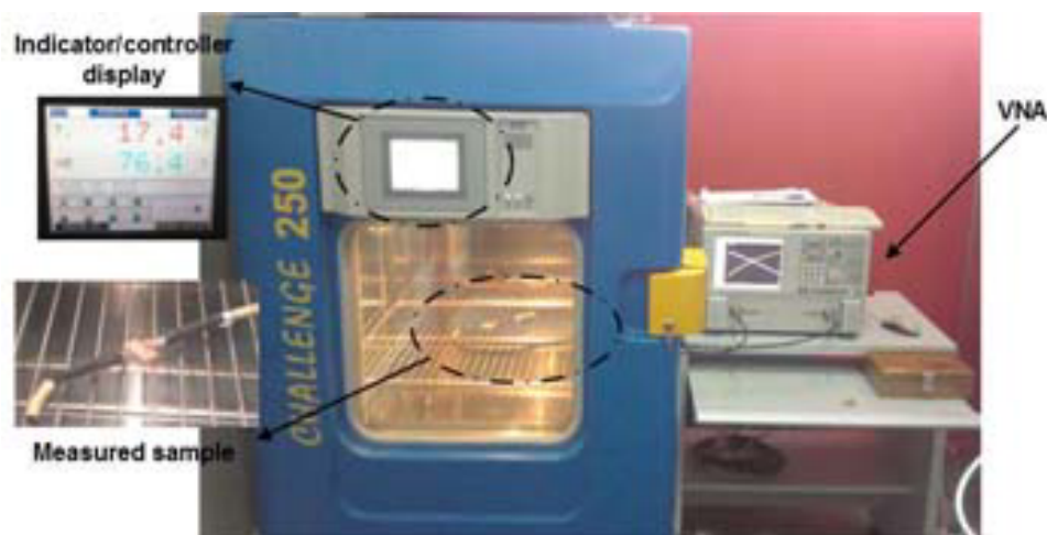
Figure 1.7: Climatic chamber measurement setup
