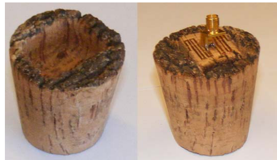
Figure 2.33: (left) - barrel cork stopper with the hole. (right) - cube antenna inside the cork stopper
