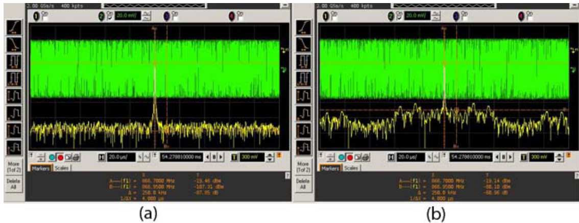
Figure 5.13: (a) tag no response - (b) tag response
