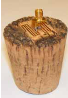
Figure 5.9: Photograph of the antenna inside a cork stopper
