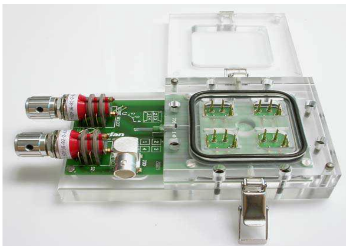
Figure 25: Solar Cells holding device for measuring the characteristics of the solar cells
