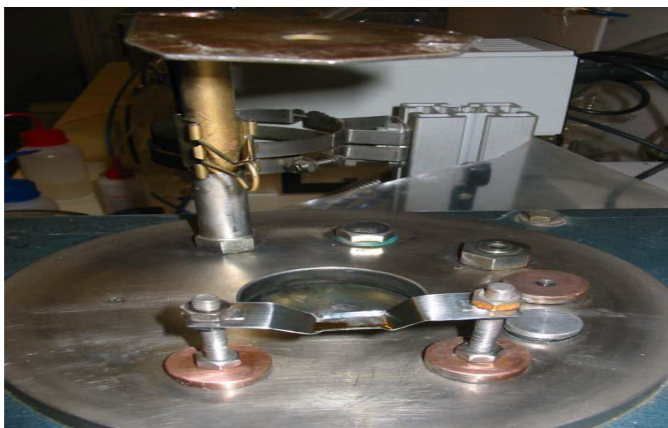
Figure 22: the metal evaporation boats and the substrate holder on top.
