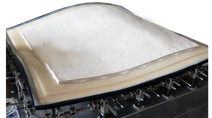
[fig.90] Adaptive Mould Machine. Aalborg, Dinamarca. Adapa, 2010.
