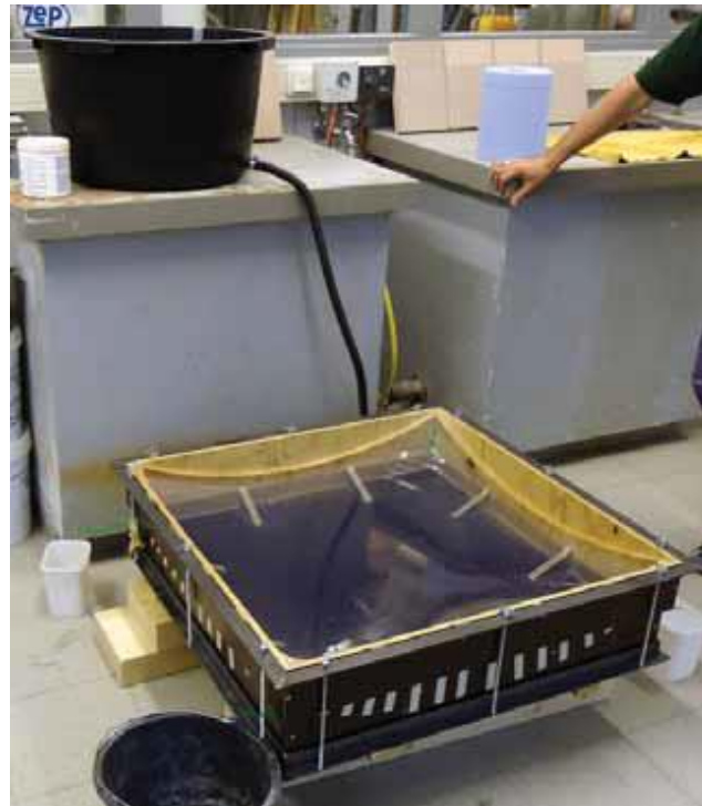
[fig.88] Fabric Formwork. Eindhoven, Países Bajos. Rob Verhaegh; Eindhoven University of Technology, 2010.
