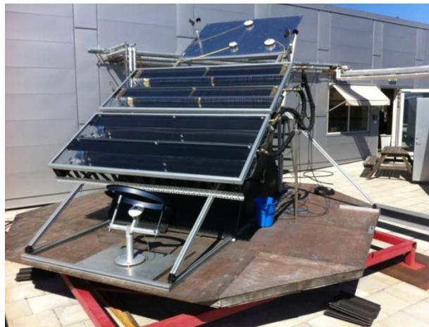
Figure 7.1: Picture shows how the PV-T and the T-collectors were installed
