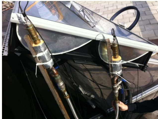
Figure 7.3: Collector inlet side with Pt 100 sensors inside
