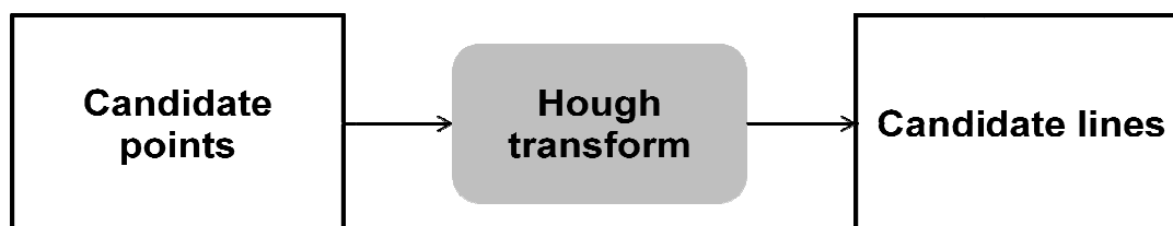
Fig. 3. 9: Input and output of the Hough transform.
