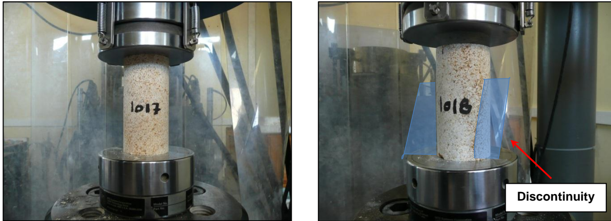
Figure 3-24. Uniaxial compression test.
