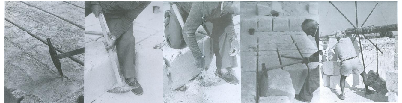
Fig.18. Traditional process of manual extraction of sandstone
