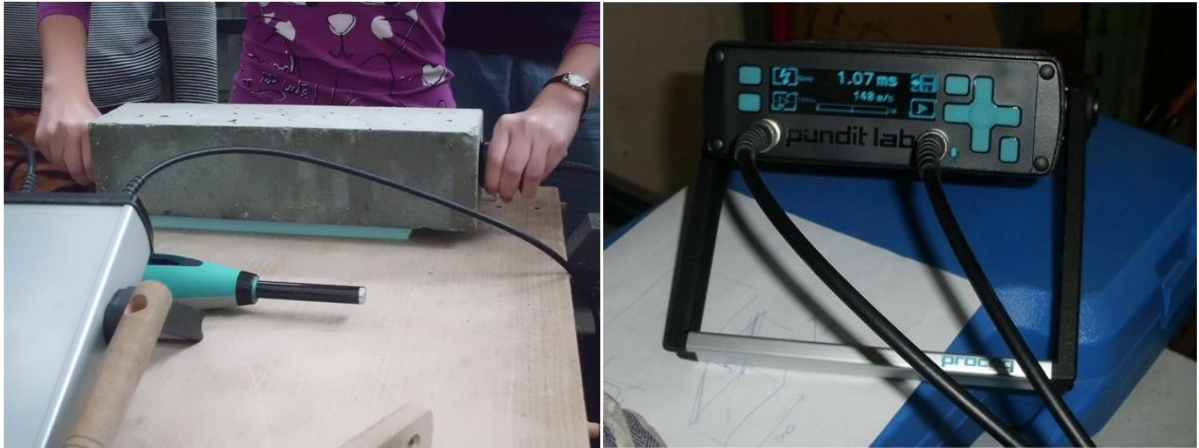
Figure 4.5 Procedure of the pulse velocity method
