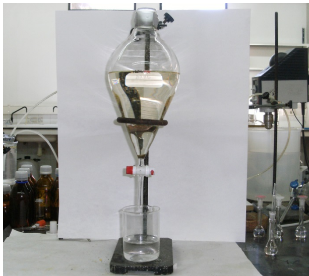
Fig. 3 : Separator filled with organic phase after shaking, aqueous phase already withdrawn into the beaker
