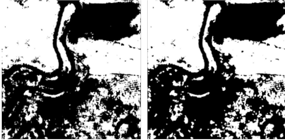
Figure 5.11: Right: Tree band after the noise removing process. Left: Result of applying an opening with a disc-shaped structuring element of diameter 15 on the image on the right.
