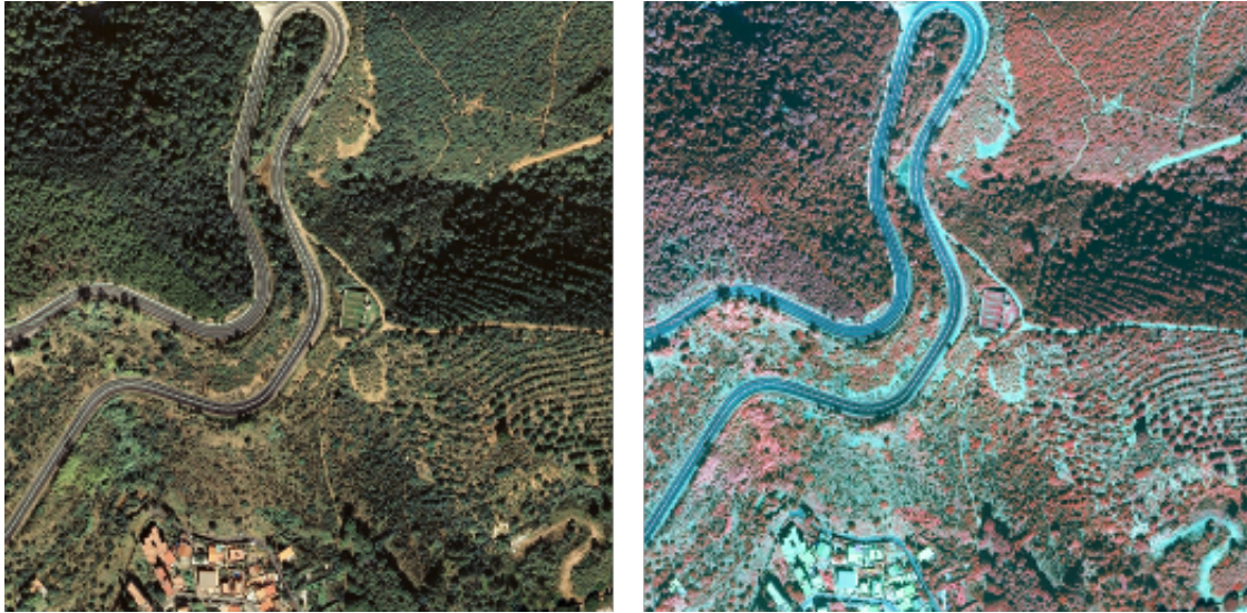
Figure 4.3: ©Cartographic base orthophoto property of the Institut Cartogràfic de Catalunya, available on www.icc.cat [1]. Left: RGB orthophoto. Right: Orthophoto with infrared information coded in the R channel, red information coded in the G channel and green information coded in the B channel..
