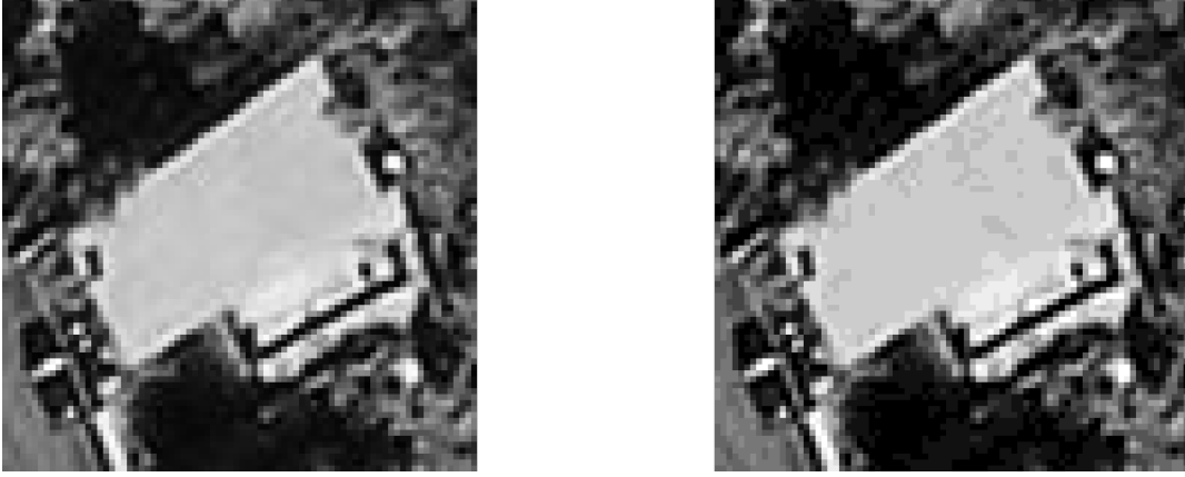
Figure 4.6: Left: Aerial image extracted from ICC[1]. Right: Image on the left discretized using 16 grey values.
