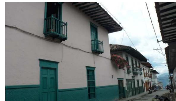
Figure 3.14. Typical housing in cemented bahareque. Salamina. Personal document.
