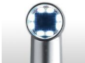
Fig.5.38. Digital Endoscope with CMOS image sensor placed at the tip (Source: Yole)
