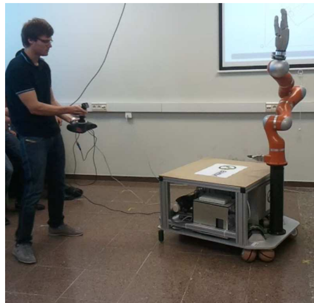
(d) The platform controlled by the joystick.
