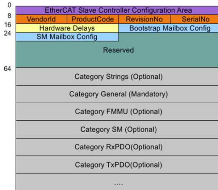
Figure A.4: Slave EPROM structure
