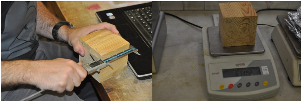
Illustration 25: Measured and weight of the specimens
