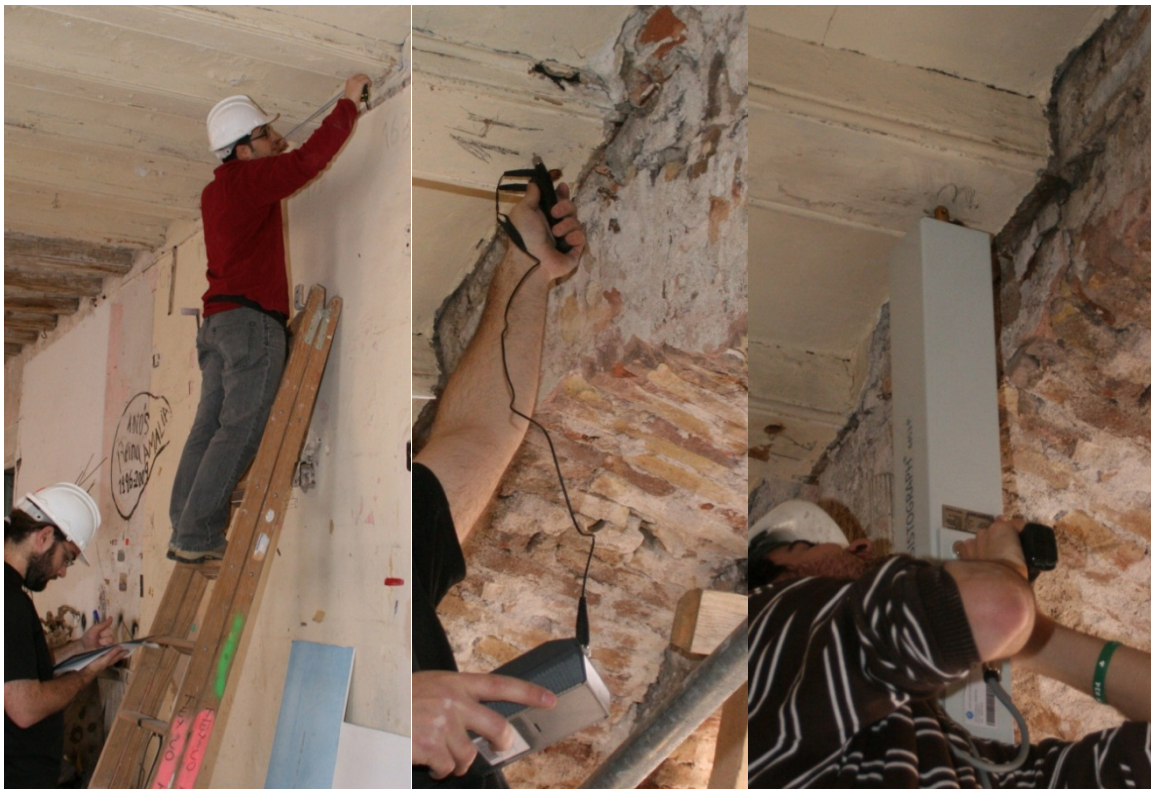
Illustration 4: Register of beams geometry. Humidity of beams. Assay with the Resistograph
