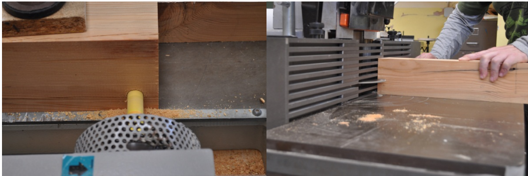
Illustration 27: Preparing micro specimens
