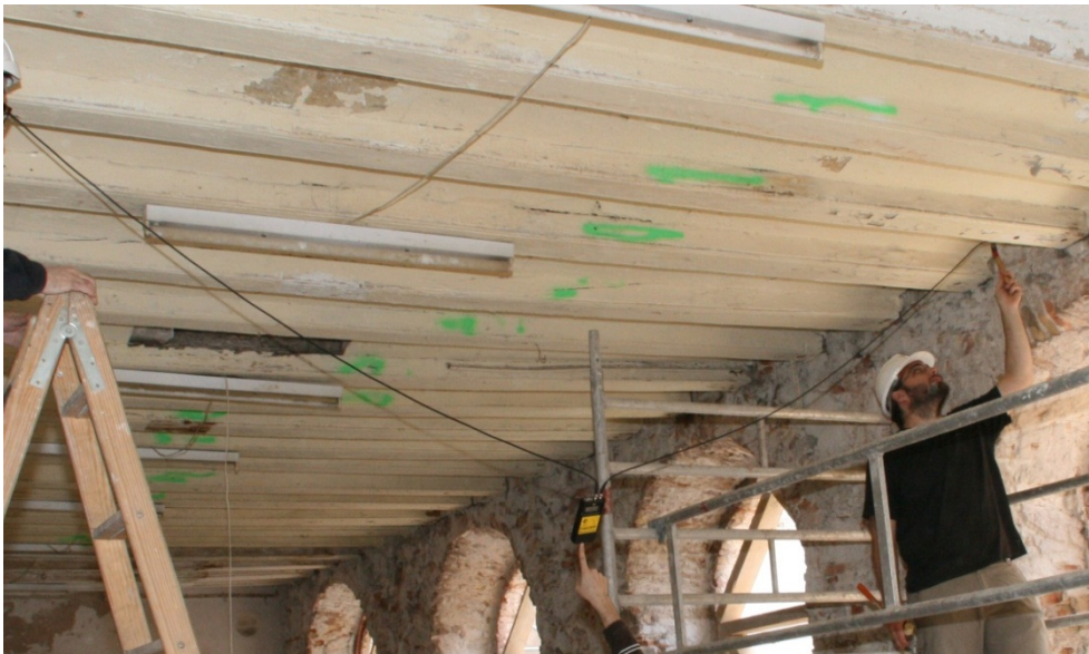
Illustration 6: General view of acoustic assay of the waves of impact
