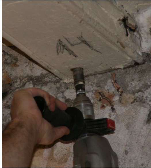
Illustration 5: Extraction of cylindrical micro samples
