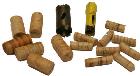
Illustration 26: Drill bit and micro specimens
