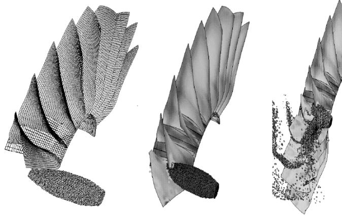
Figure 6.5: An application in aeronautics. Bird strike simulation. See [2].
