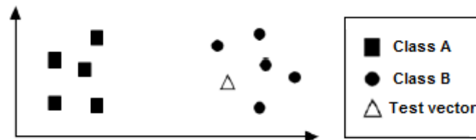
Figure 2.11- Image illustrating two different classes and a test class which has to be classified.
