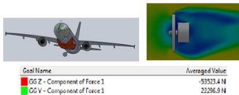
Fig. 4. 21 Lift (green) and Drag (red) values for RAT in the nose and tail at sea level
