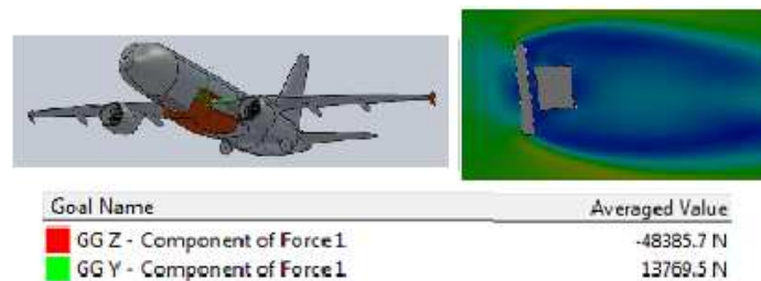
Fig. 4. 16 Lift (green) and Drag (red) values for RAT in the tail at sea level
