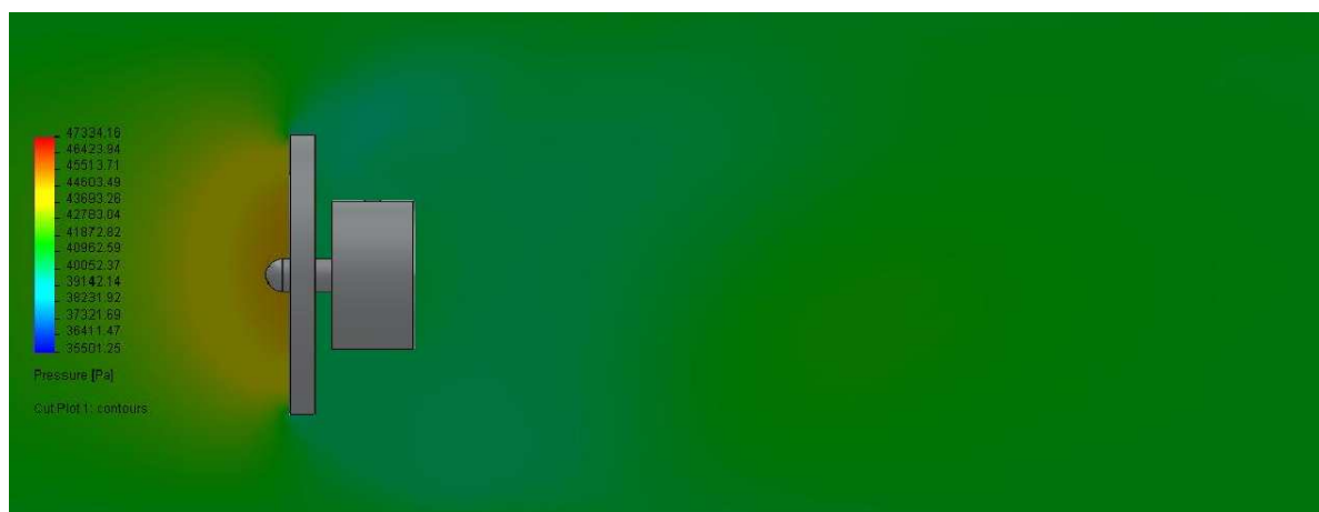
Fig. D. 21 Pressure simulation with the RAT in the nose at 7,000 ft in detail
