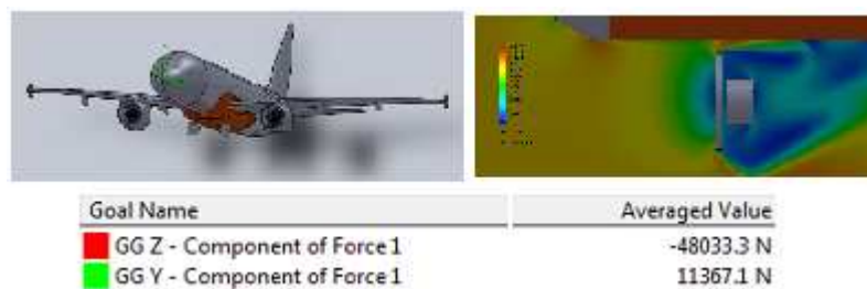
Fig. 4. 24 Lift (green) and Drag (red) values for RAT in the belly-fairing at 7,000 ft
