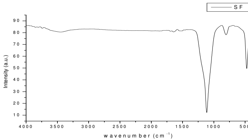
Figure 17 Fourier Transform Infra-Red for the silica fume.
