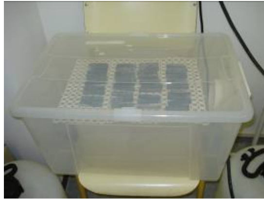
Figure 21 Samples at carbonation chambers.
