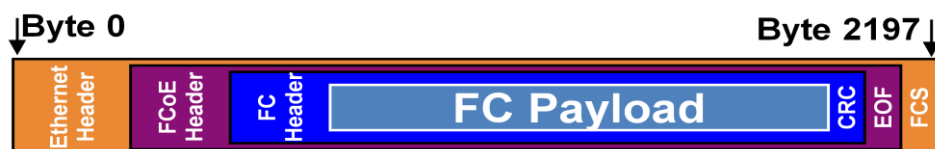
Fig. 2.3 Encapsulated package using FCoE
