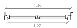
FINESTRA FE4 06 U (130x120) MATERIAL : ALUMINI VIDRE 3+3/6/3+3 AGAFADORS/PANY : MANETES OBERTURA : 2 FULLES OSCILLOBATENTS
