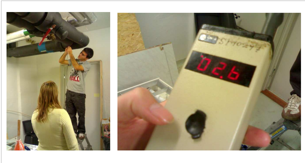
Figure 4.3.1: Measurements performed with the KrautKramer DM2 thickness gauge.
