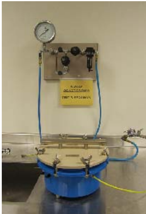
Fig.2.25 – Esquema Pressure Plate
