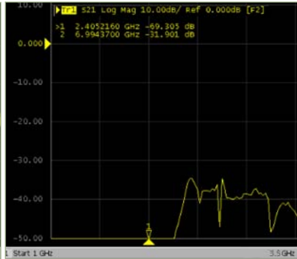
Figure 38. Power received by the coke can when both antennas are pointing to the roof
