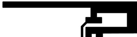
Figure 9. Shape of the DN007 antenna reference design
