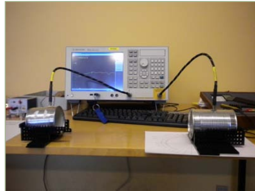
Figure 36. Way to measure the radiation pattern of the waveguide
