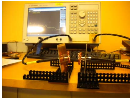
Figure 28. Configuration to measure the radiation pattern of two Biquad antennas.
