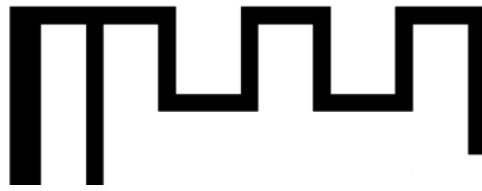
Figure 8. Shape of the ANo43 antenna reference design
