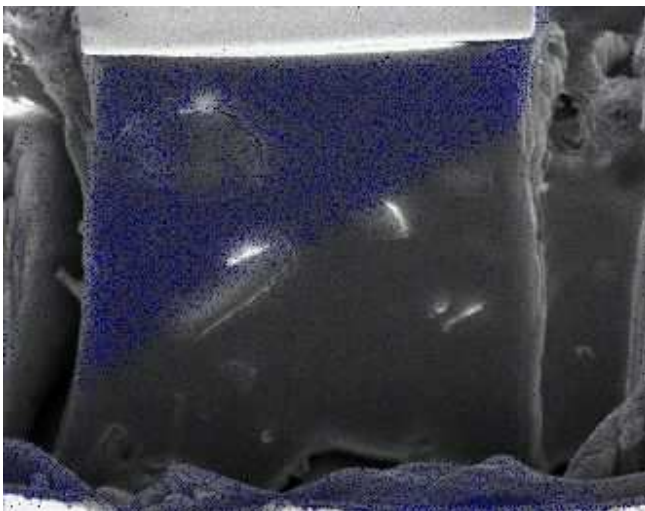
Figure 10. Figure 9 with a mapping test to illustrate the location of Fe (dark blue).
