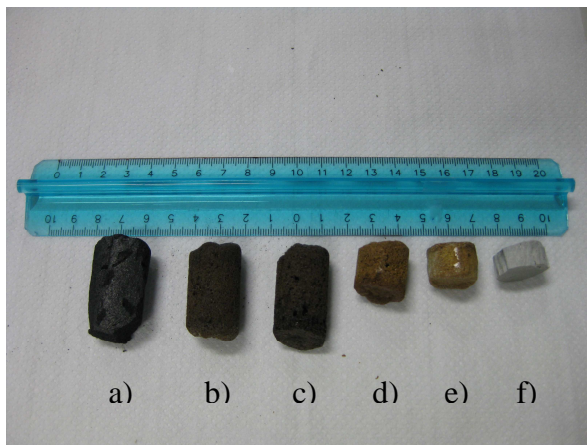
Figure 10 Degraded epoxidic resin at: a) 800°C, b) 600°C, c) 400°C, d) 350°C, e) 325°C, f) non-degraded
