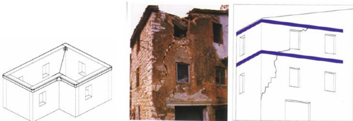
Figure 5.2.6.3 External circumferential tie-rods: a) metallic elements, b) FRP or other composites (Blasi et al. 1999)
