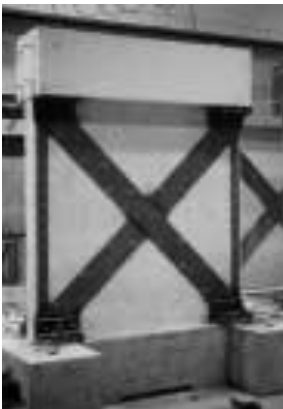
Figure 5.2.7.28 (a) Using vertical and diagonal bracing panel (reproduced after Rai and Goel 1996) (Taghdi 2000)
