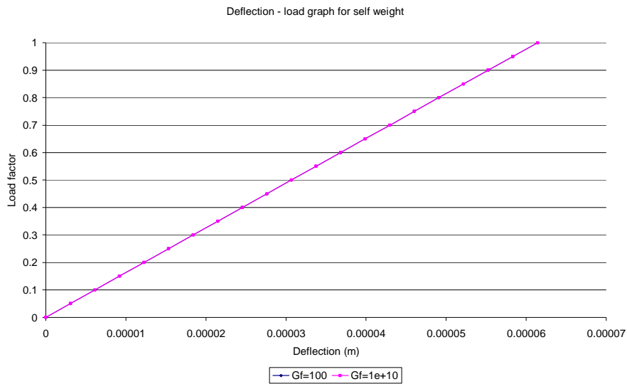
Figure 3.13 - Deflection – load factor for self weight
