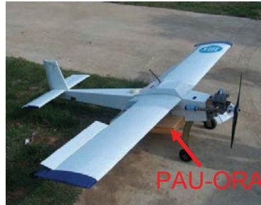
(b) PAU-One Receiver Airborne instrument block mounted on the bay of a Remote Control aircraft.
