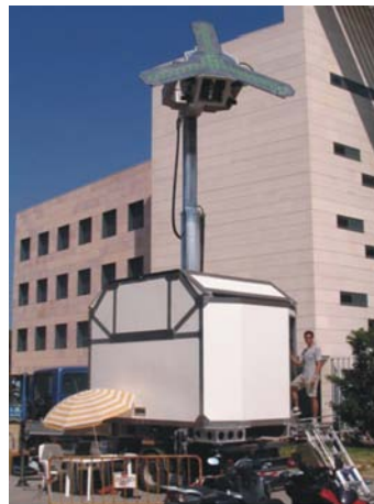
(d) PAU-Synthetic Aperture. View of the whole instrument installed on truck with 8 m robotic mast.
