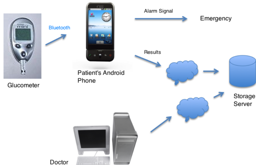
Figure 4.1: Architecture of GlucoServer
