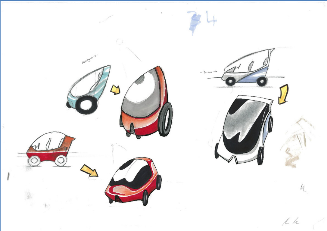
Figure 7.19: New sketches combining aerodynamic shape with efficient size and weight
