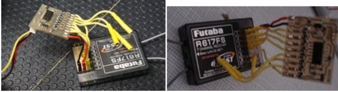
Figure 3.24 Proper connection of the Receiver with the MeekPE Encoder
