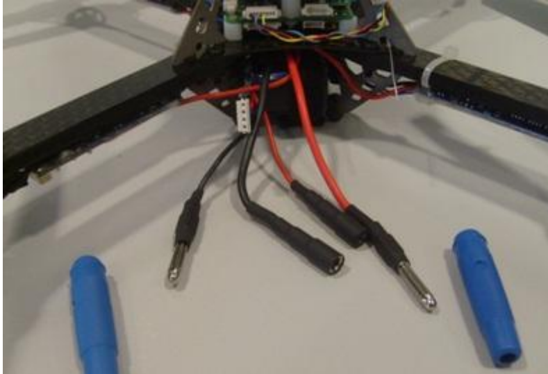
Figure 3.17 Connectors between Battery and Power Supply
