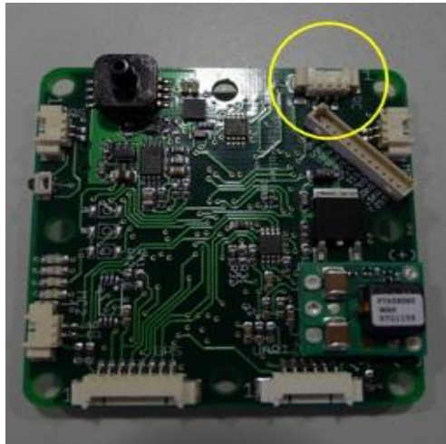
Figure 3.15 Location of the RC connector in the Main Board
