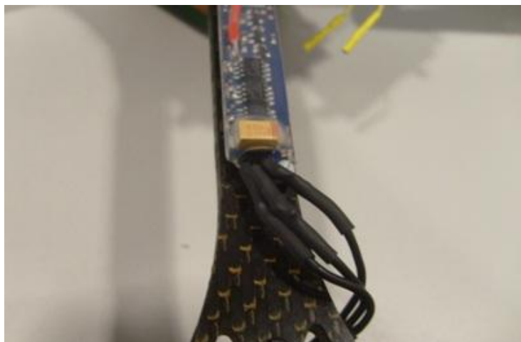
Figure 3.20 Connection between the Controllers and the Engines
