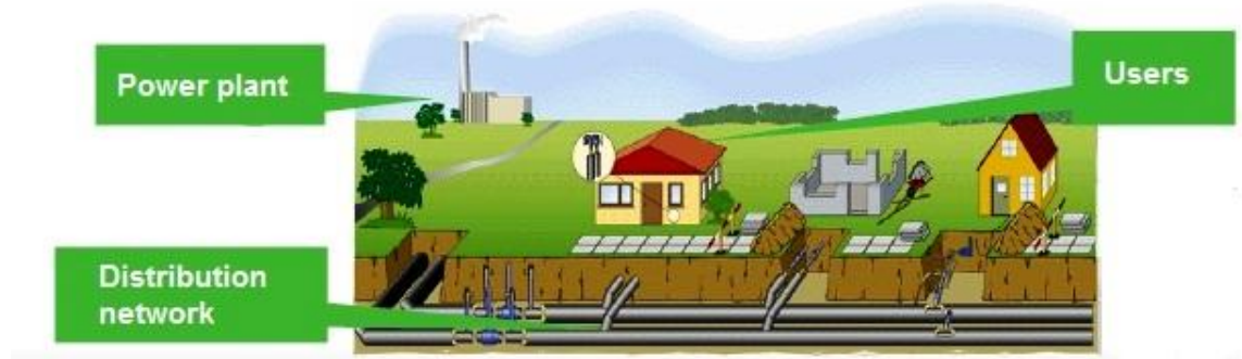
FIGURE 33. Main parts of district heating and cooling.
