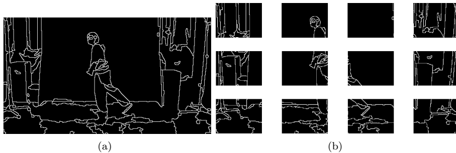
Figure 2.5: Sub-imaging example. (a) Edglets computed from the original image, taken from the Watershed algorithm result, (b) 12 sub-image division.
