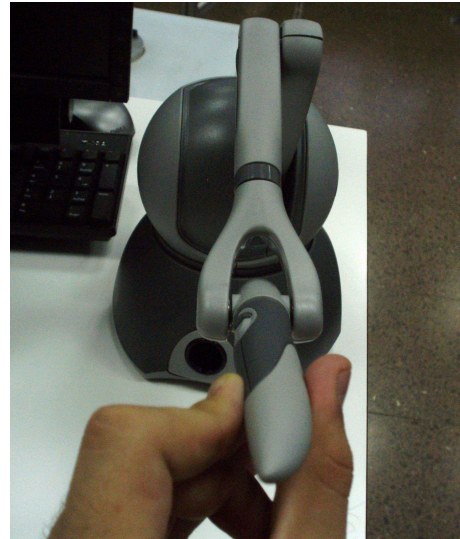
(b) To obtain the result shown in the picture A.5(a) the 6 th joint of the device has to be rotated counterclockwise as shown.
