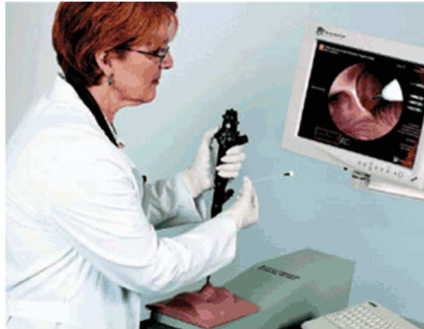
Figure 2.3: The VR bronchoscopy skill station includes a cart, computer, display, printer, proxy flexible bronchoscope, and keyboard. While the operator performs Flexible Fiber Bronchoscope via the left nares, realistic resistance is felt during manipulation of the proxy flexible bronchoscope.
