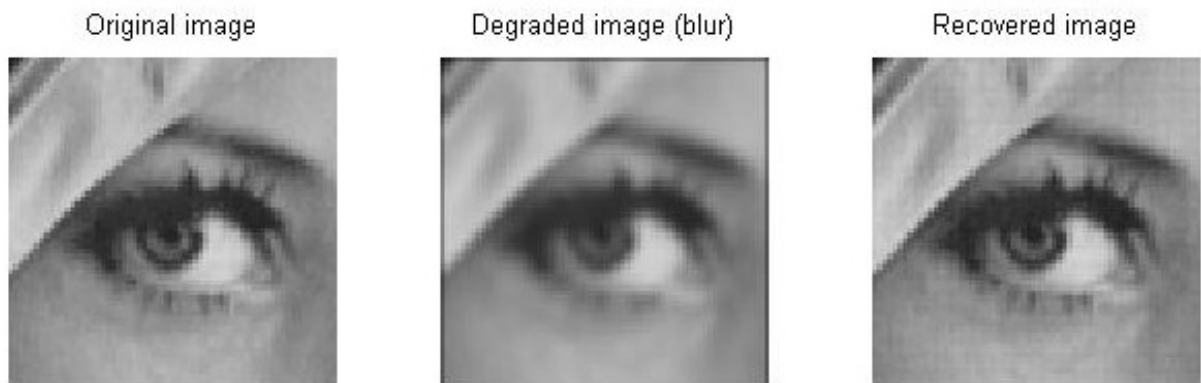
Figure 1.1. Original image to be reconstructed, degraded (blurred) image and recovered image using the inverse matrix reconstruction method developed in the project
