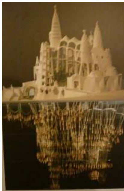
Figure 2.12 Gaudi 's hanging hanging model for the crypt of the chapel of the Colonia Güell 1898-1919 compared with a model of the geometry of the structure (museum of Sagrada Familia at Barcelona, Spain)
