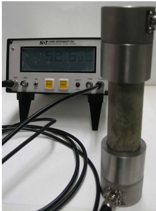
Figure 4.7 Ultrasonic pulse test equipment and sample.
