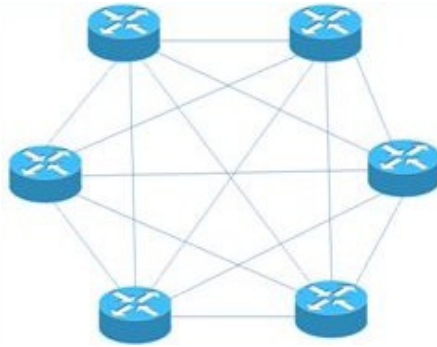
Figure 6.3 - Interconnection of 6 core routers into a full mesh topology using 15 direct IP links
