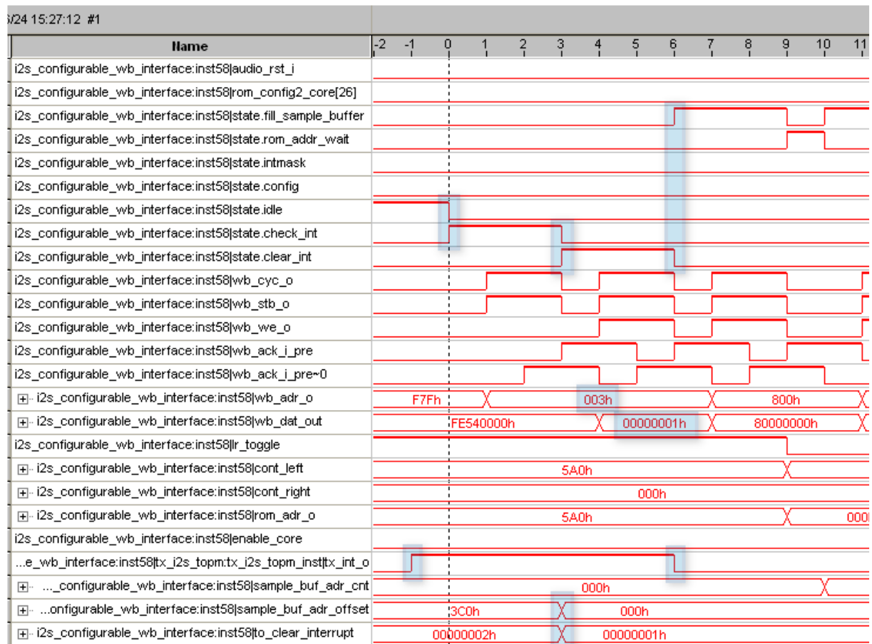
Figure 9.34. Timing diagram of core signals and state transitions during interrupt handling
