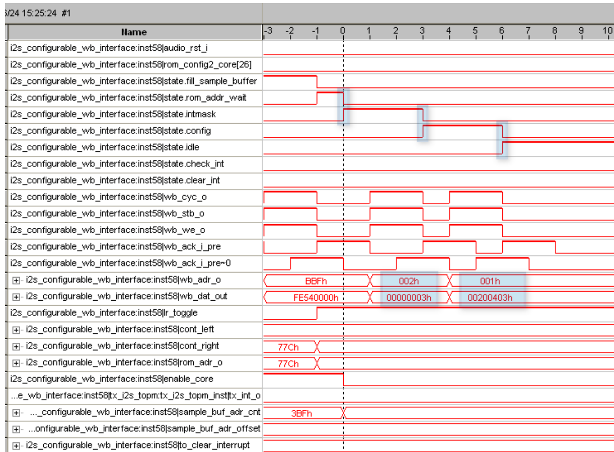
Figure 9.33. Timing diagram of core signals and state transitions during initial configuration
