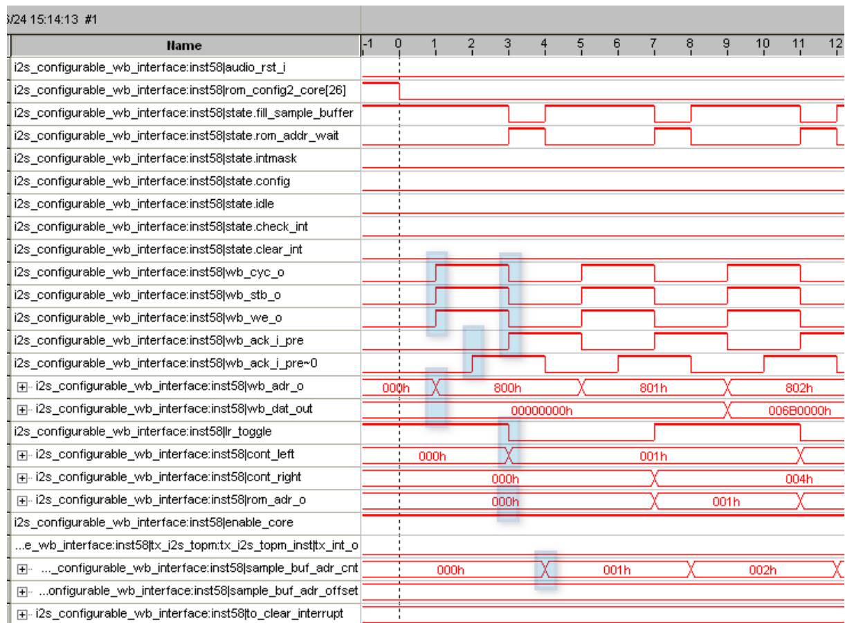
Figure 9.31. Timing diagram during FILL SAMPLE BUFFER state just after a full reset
