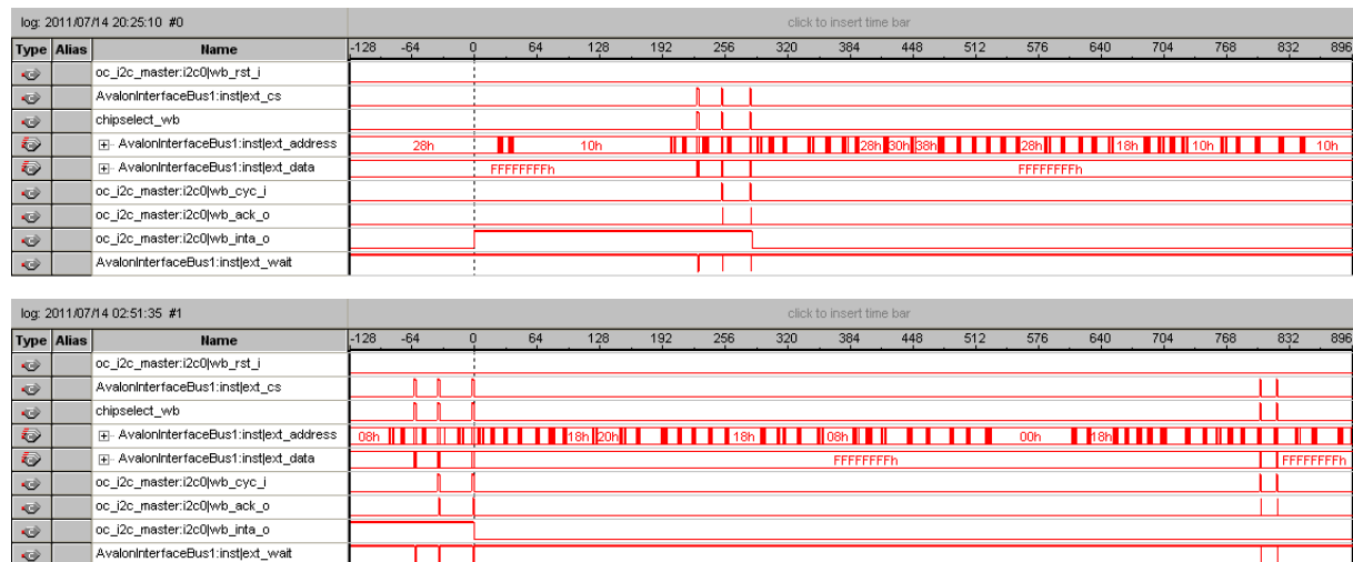
Figure 10.4. SignalTap captures showing time needed to clear the interrupt and idle time until core is configured with next data to send for ISR method
