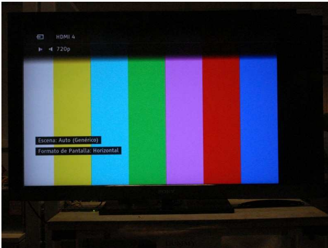
Figure 11.21. Default 720p Color Bar pattern from HDMI generator in test TV screen
