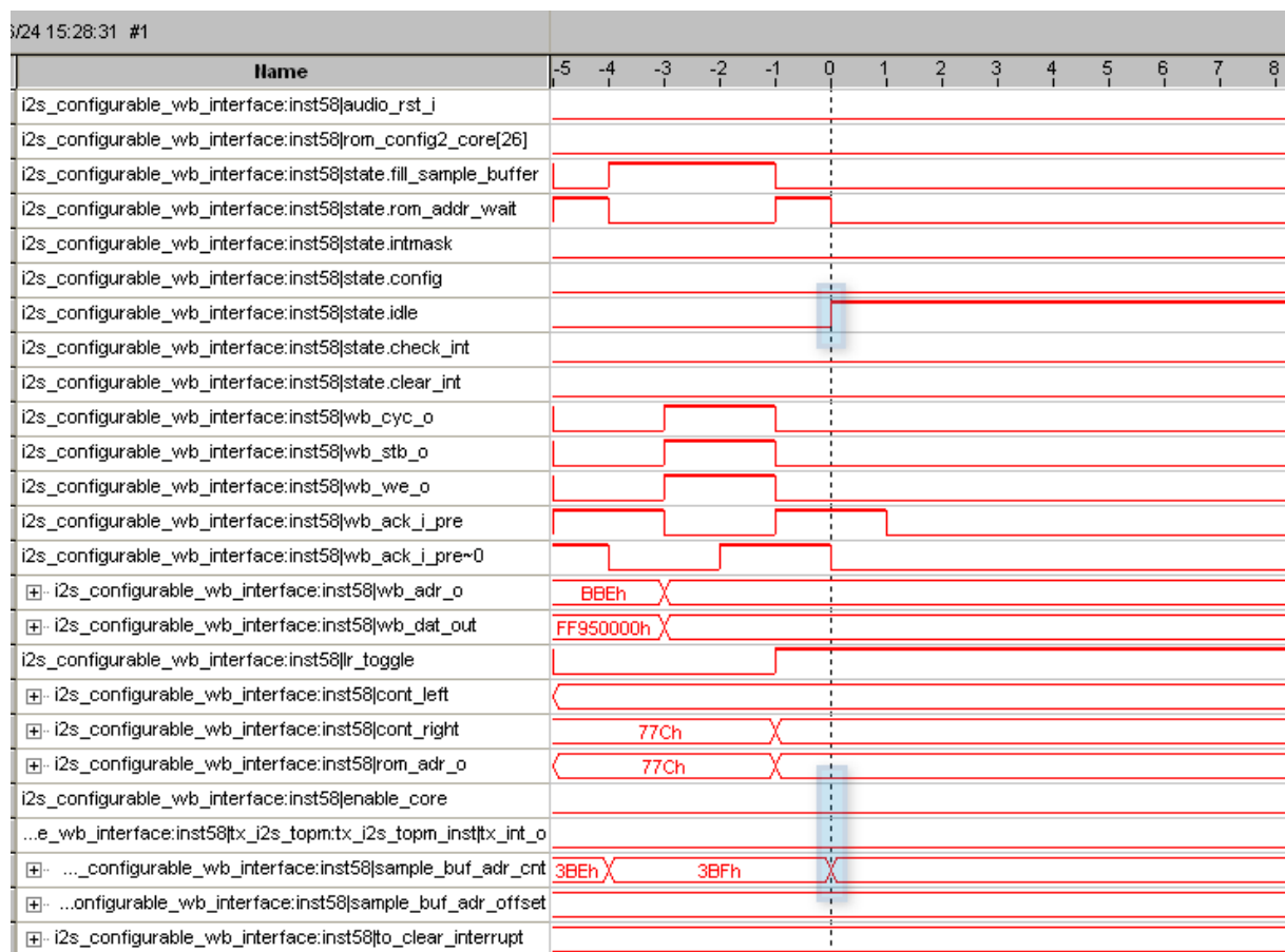
Figure 9.32. Timing diagram of core signals when leaving FILL SAMPLE BUFFER state
