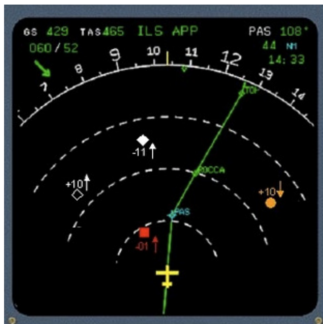
Figure 1: Display of TCAS system situated in the cockpit
