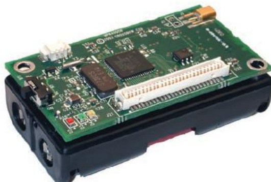
Figure 1-3 A rectangular MICA mote
