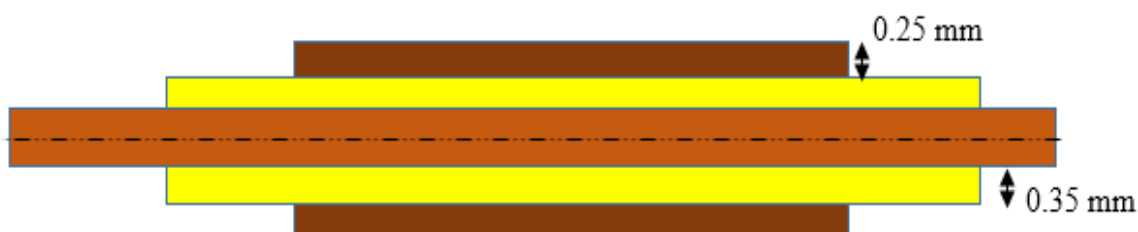
Figure 3.18 Geometry of model with shield length 50% of electrode length. Physical dimensions of the model are as shown above. The yellow color indicates a dielectric material of permittivity 2.1. Brown color indicates a metallic conductor.
