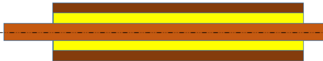
Figure 3.19 Geometry of model with complete shield length (i) 90% of electrode length for electrode length of 12.5 cm (ii) 95.2% of electrode length for electrode length of 25 cm.
