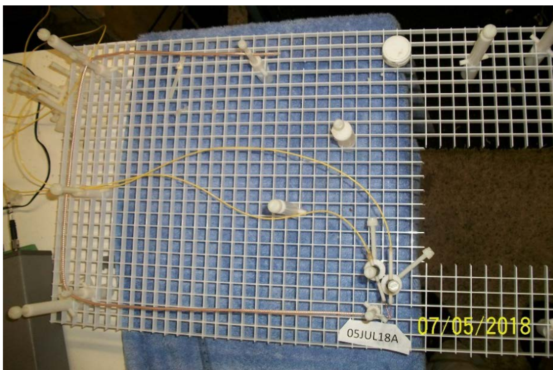
Figure 5.19 Pathway for 80 cm RG 316 coaxial cable that serves as a model lead. The same pathway was used for all of the tests on the 80-cm long structures
