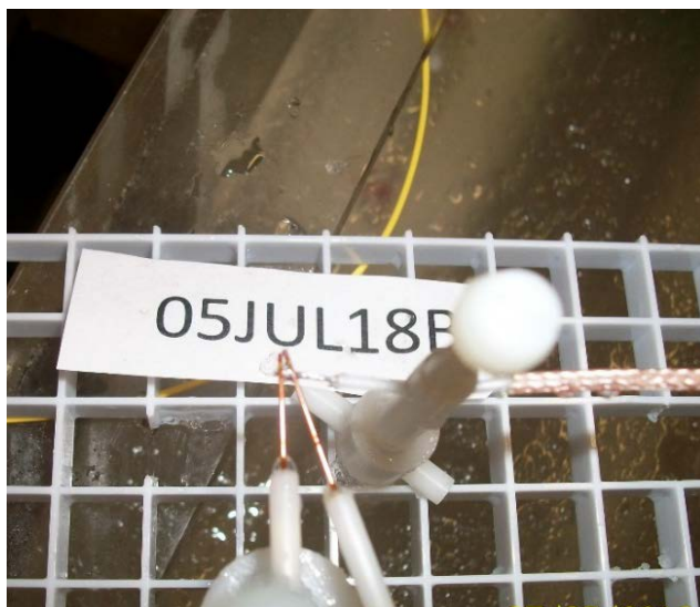
(c) Neoptix probe in contact with an electrode of the model implant (left) and phantom with the model implant kept in an MR coil (right)
