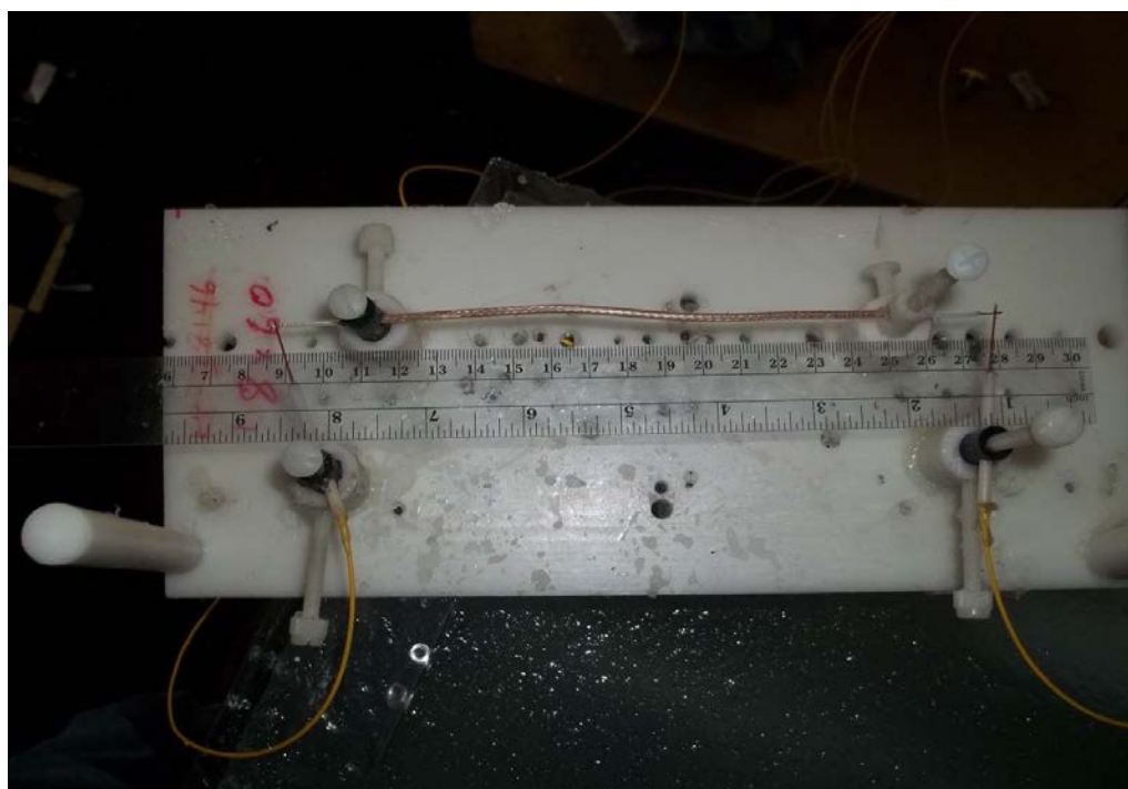
Figure 3.12 Temperature probe placement on 20 cm shielded model lead. Length of the shield is 16 cm. Probes are on the distal and proximal ends.
