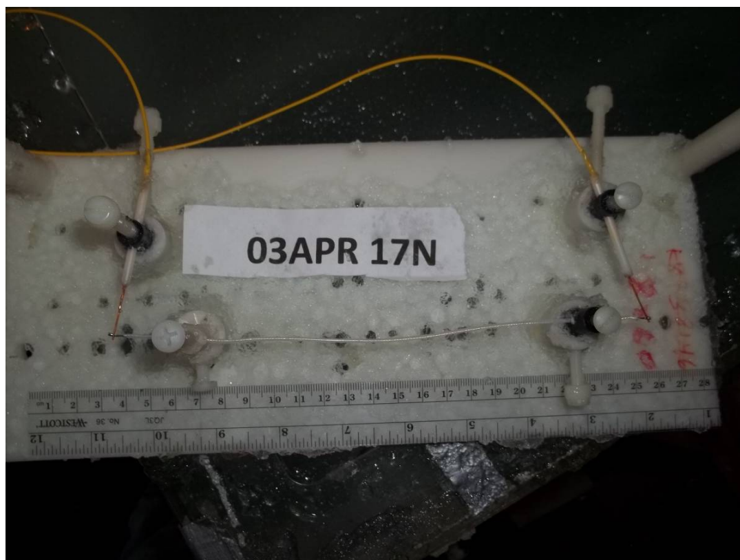
Figure 3.13 Temperature probe placement on 20 cm shielded model lead. Probes are on the distal and proximal ends
