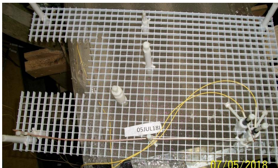
Figure 5.22. Pathway for the 45-cm insulated inner conductor of RG 316. The same pathway was used for all of the tests on the 80-cm long structures.
