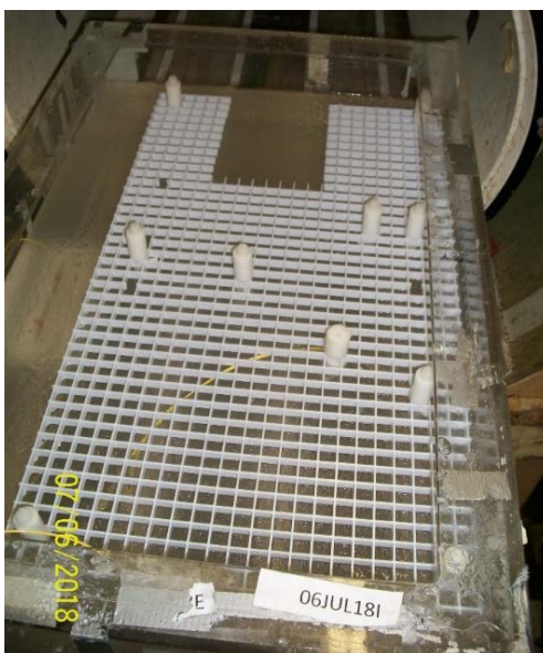
Figure 7.16 Pathway for Model 303 Cyberonics lead for temperature measurement. The same pathway was used for all of the tests on the various configurations for Cyberonics lead. Also shown, is the Cyberonics lead with Neoptix cables placed on the plastic mat. The plastic mat is kept in phantom that goes inside MRI coil.
