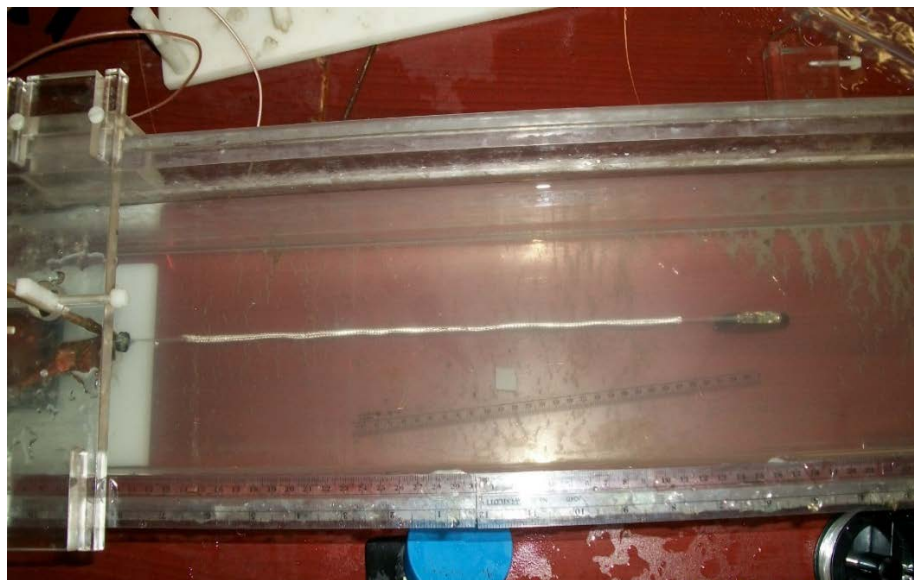
Figure 7.2 Setup to measure electric field transfer function for Cyberonics lead
