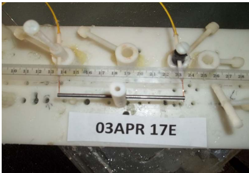
Figure 3.11 Temperature probe placement on Ti grade V rod for SAR calculations. Probes are at distal and proximal ends.
