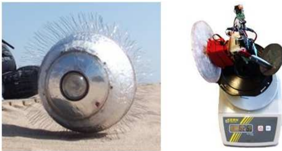
Figure 6 a) Pico-Rover on the beach and b) Less than 1 kilogram component
