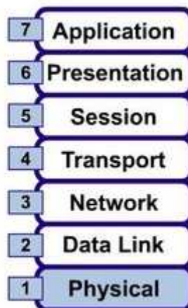
Figure 8 OSI layered structure
