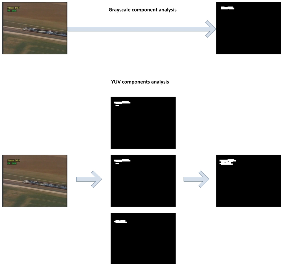
Figure 4.3: Haar Power Masks - Haar Power Mask based on the Haar wavelet decomposition of the grayscale image( upper block ) and 3 channels of the YUV image (lower block)
