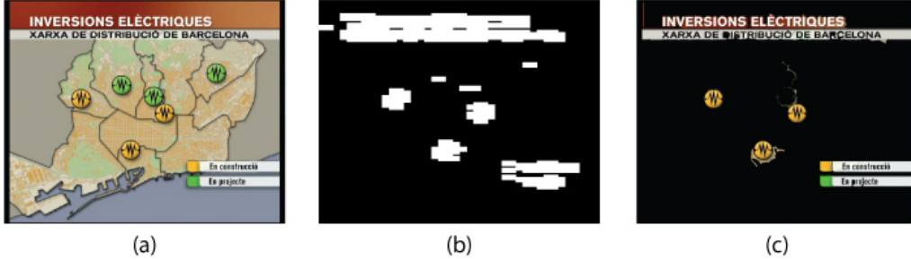
Figure 4.4: Regions selected based on Haar power mask - (a)Original image, (b)Mask based on power of HL and LH subbands of Haar wavelet decomposition, (c)Regions of the search partition which are selected, based on mask from (b)
