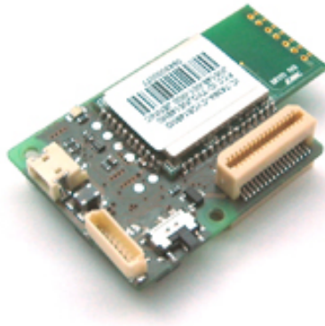
Figure 2.3: iSense core module - contains the processing unit, radio, timer and clock
