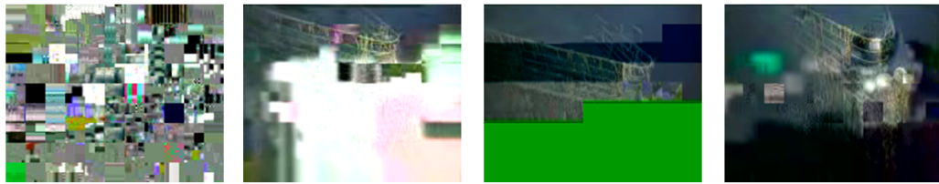
Figure 6.12: Damaged frames due to sudden changes in the speed between the transmitter and the receiver.
