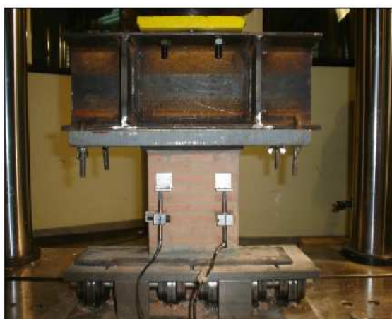
Figure 39: Prism specimen under test.
