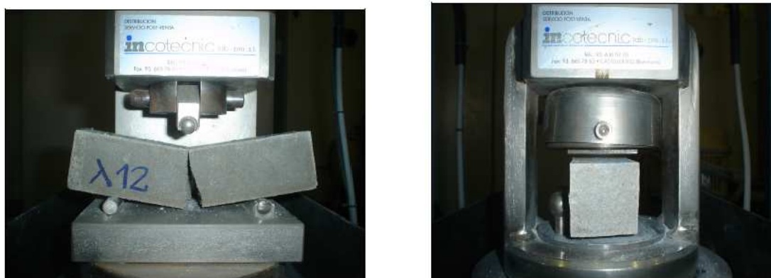
Figure 37: Flexural strength test of mortar (left) compressive strength test of mortar (right).
