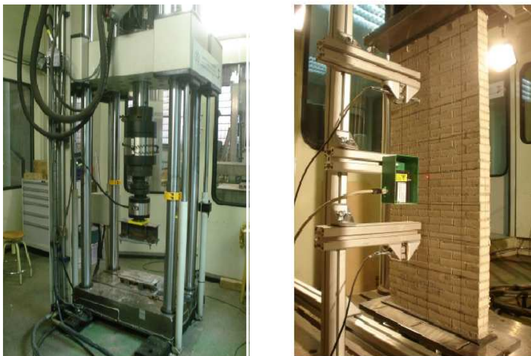
Figure 42: Press INSTRON machine for compression and Young's modulus test (left) and Laser scanner for measurement of displacement (right).
