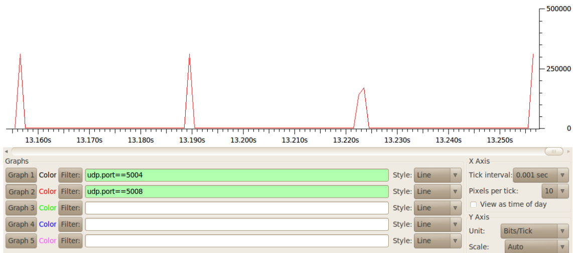
Fig. 4.5 Graphical timing Wireshark captured packets. 6 audio channels
