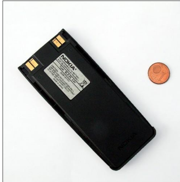
Illustration 61 Lithium polymer battery from a Nokia cell phone. Picture taken from http://pl.wikipedia.org/wiki/Plik:Lipolyo1rp.jpg
