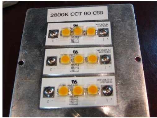
Illustration 37 Light creates a warm white light with LEDs that have Nanosys' material layered over them Picture taken from http://www.treehugger.com/files/2010/01/ces-2010-nanosys-using-nanotechnology-to-make-led-lighting-more-beautiful.php
