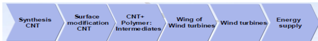
Illustration 24 Schematic process since it is synthesized nanomaterial until applied to the turbine
